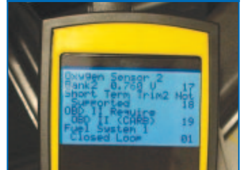
Figure 2: Make sure your scan tool can handle data from a wide range A/F sensor. This generic OBD II scanner reported PIDs for both conventional rear O 2 sensors, but had nothing to say about the front two wide range A/F sensors.
