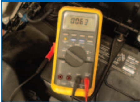
Figure 1: After providing power to the A/F sensor heater, we attached a DVOM to the two other sensor leads. After starting the engine, the sensor responded like a conventional O 2 sensor.
